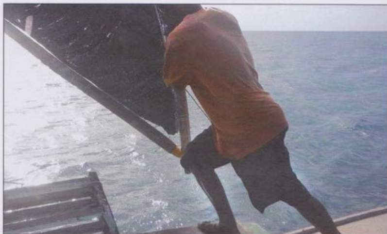
Tacking a Marshallese canoe involves releasing the downhaul on the sprit and boom and moving the tack from the bow to the stern—which, respectively, become the new stern and the new bow. Here, Taidik Mae moves the sprit to the new bow while changing tacks.
